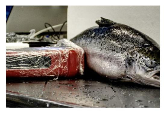
Figure 24 Measurement of pigmentation from whole dead fish with handheld SORS instrument.
